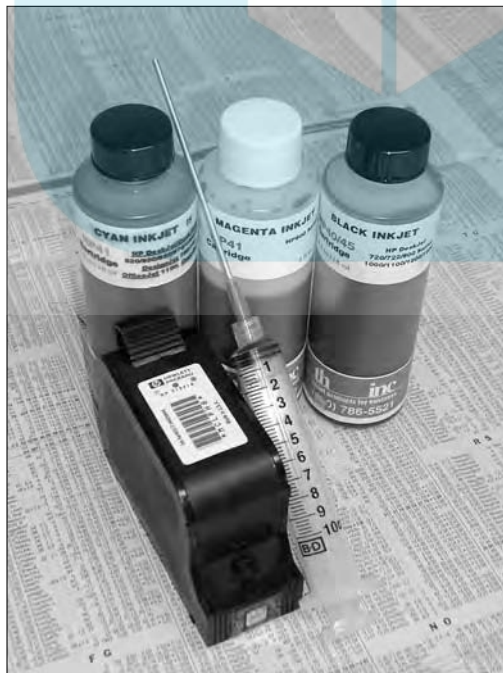
Figure 4-6: Many companies sell refill kits to extend the life of inkjet cartridges.
